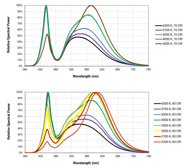
The following graphs are the result of a series of pulsed measurements at 1400 mA and  $T_{J}$  = 85 °C.
