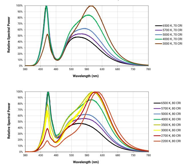
The following graphs are the result of a series of pulsed measurements at 990 mA and T<sub>1</sub> = 85 °C.
