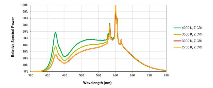
The following graphs are the result of a series of pulsed measurements at 1620 mA and  $T_{\rm _J}$  = 85 °C.
