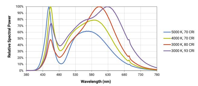
The following graph is the result of a series of pulsed measurements at 550 mA and TJ = 85 °C.
