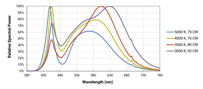
The following graph is the result of a series of pulsed measurements at 550 mA and TJ = 85  $^{\circ}$ C.
