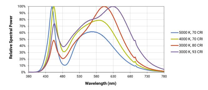
The following graph is the result of a series of pulsed measurements at 1100 mA and  $T_{_{\rm J}}$  = 85 °C.
