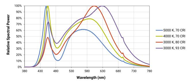
The following graph is the result of a series of pulsed measurements at 1900 mA and  $T_{\rm _J}$  = 85 °C.
