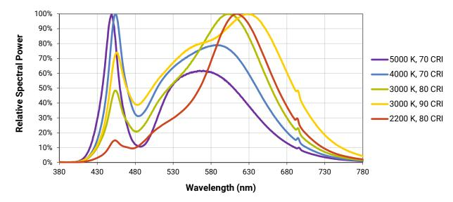
The following graph is the result of a series of pulsed measurements at 800 mA and  $T_J$  = 85 °C.
