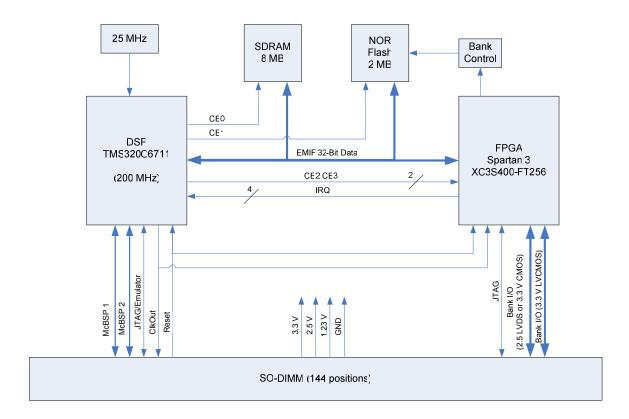
Figure 1 MityDSP Block Diagram
