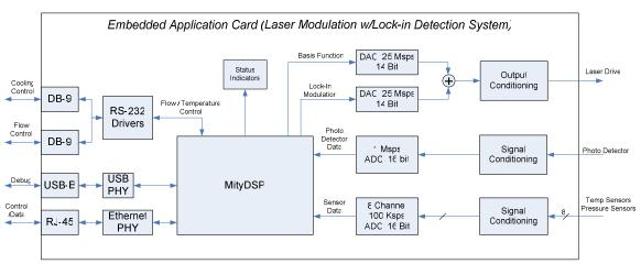
Figure 2 Typical MityDSP Application
