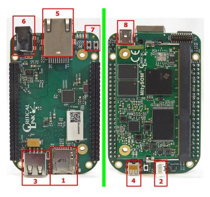
By default the MitySOM-335x Maker Transition Kit is configured to boot from the included MicroSD card. Make sure that the MicroSD card has been inserted fully into the slot, J401 (Find 1).
