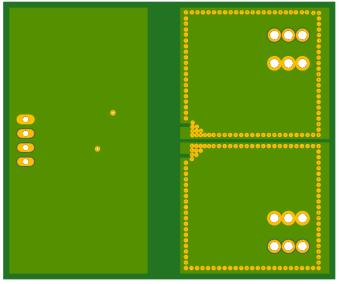
Figure 42. Recommended PCB Layout (Bottom Layer) for the 20 A to 65 A variants of the CT426.
