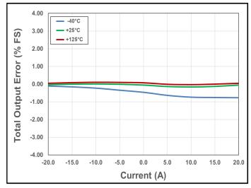
Figure 14. Total Output Error vs. Current vs. Temperature
