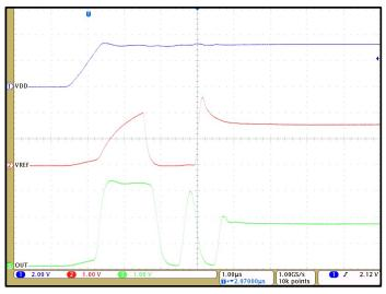
Figure 6. CT426 Startup Waveforms for  $V_{OQ}$  = 1.65 V (AC Current)
