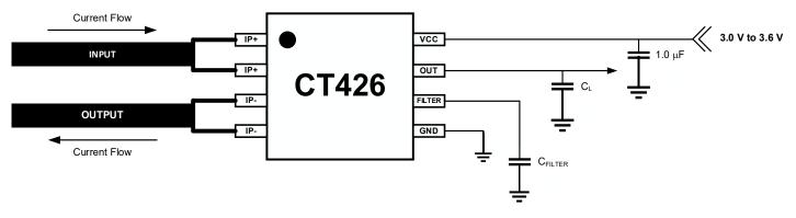
Figure 40. CT426 Application Block Diagram
