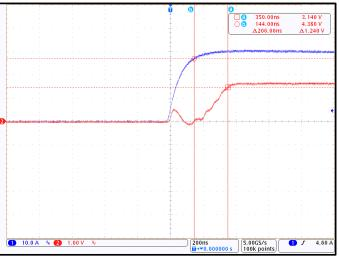
Figure 8. CT426 Response Time;  $I_{P}$  = 30  $A_{PK}$  and  $C_{L}$  = 100 pF
