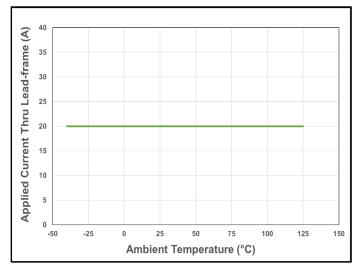
Figure 13. CT426 Current De-rating Curve for 20  $A_{\text{DC}}$
