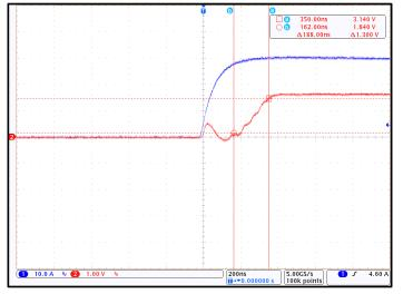
Figure 9. CT426 Rise Time;  $I_{\text{P}}$  = 30  $A_{\text{PK}}$  and  $C_{\text{L}}$  = 100 pF
