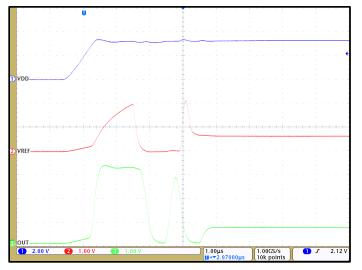
Figure 5. CT426 Startup Waveforms for  $V_{OQ}$  = 0.65
