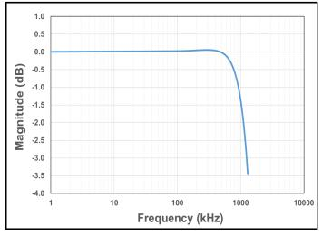
Figure 7. CT426 Bandwidth with C<sub>FILTER</sub> = 1.0 pF
