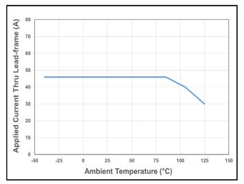
Figure 34. CT426 Current De-rating Curve for 65  $A_{\text{PK}}$  (46.0  $A_{\text{DC}})$
