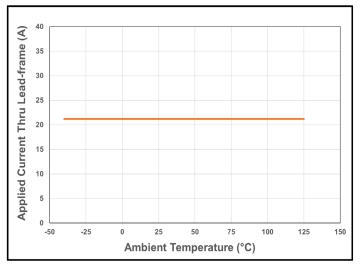
Figure 22. CT426 Current De-rating Curve for 30  $A_{\text{PK}}$  (21.2  $A_{\text{DC}})$
