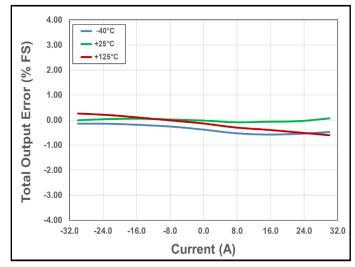
Figure 20. Total Output Error vs. Current vs. Temperature
