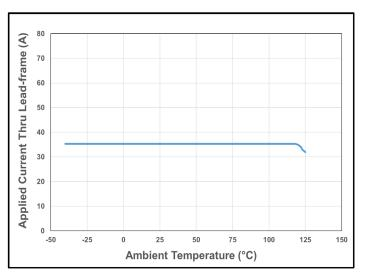
Figure 28. CT426 Current De-rating Curve for 50  $A_{\text{PK}}$  (35.4  $A_{\text{DC}})$
