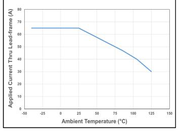
Figure 31. CT426 Current De-rating Curve for 65 A<sub>DC</sub>
