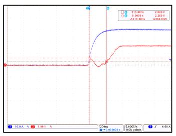
Figure 10. CT426 Propagation Delay;  $I_{\text{P}}$  = 30  $A_{\text{PK}}$  and  $C_{\text{L}}$  = 100 pF
