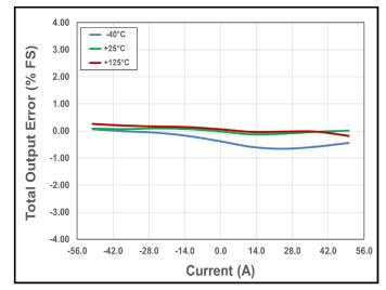
Figure 26. Total Output Error vs. Current vs. Temperature
