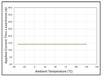
Figure 16. CT426 Current De-rating Curve for 20  $A_{\textrm{PK}}$  (14.1  $A_{\textrm{DC}})$
