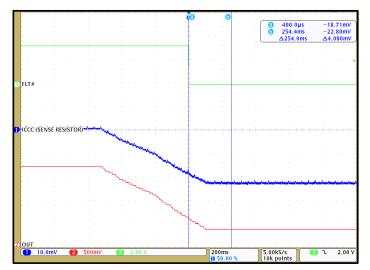
Figure 12. CT427 OCD enabled at -110% of -30  $A_{\text{PK}}$  and FLT# is LOW
