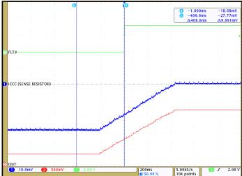
Figure 13. CT427 OCD disabled at -90% of -30  $A_{\text{PK}}$  and FLT# is HIGH
