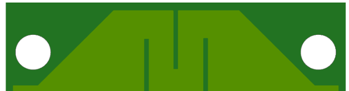
Figure 25. PCB Trace Design to Generate Differential Magnetic Field for CT452 to Measure
