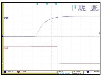
Figure 4. Power-On Time for Open Drain Output ( $V_{DD}$  and  $\overline{OUT}$ )
