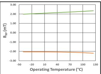
Figure 43.  $B_{RPN}$  (Orange) and  $B_{RPS}$  (Green) vs. Operating Temperature at V<sub>DD</sub> = 3.0 V
