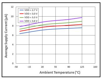
Figure 31. Average Supply Current vs. Temperature vs. Supply Voltage
