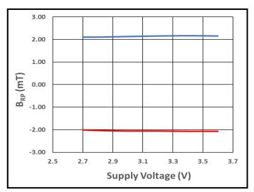
Figure 9.  $B_{RPN}$  (Red) and  $B_{RPS}$  (Blue) vs. Supply Voltage at +25°C
