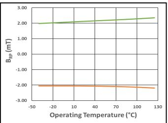
Figure 11.  $B_{RPN}$  (Orange) and  $B_{RPS}$  (Green) vs. Operating Temperature at  $V_{DD}$  = 3.0 V
