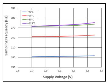
**Figure 21.** Sampling Frequency vs. Supply Voltage vs. Temperature
