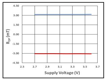
Figure 26.  $B_{\mathsf{OPN}}$  (Red) and  $~B_{\mathsf{OPS}}$  (Blue) vs. Supply Voltage at +25°C
