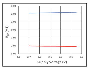
Figure 41.  $B_{RPN}$  (Red) and  $B_{RPS}$  (Blue) vs. Supply Voltage at +25°C
