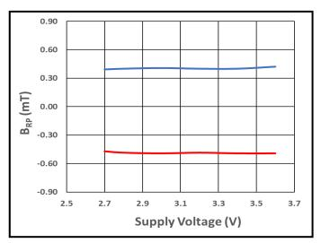
Figure 23.  $B_{RPN}$  (Red) and  $B_{RPS}$  (Blue) vs. Supply Voltage at +25°C
