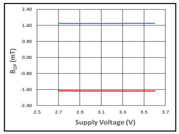
Figure 33.  $B_{\mathsf{OPN}}$  (Red) and  $~B_{\mathsf{OPS}}$  (Blue) vs. Supply Voltage at +25°C
