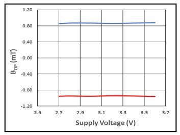
Figure 22.  $B_{\mathsf{OPN}}$  (Red) and  $~B_{\mathsf{OPS}}$  (Blue) vs. Supply Voltage at +25°C
