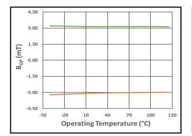
Figure 28.  $B_{OPN}$  (Orange) and  $B_{OPS}$  (Green) vs. Operating Temperature at  $V_{DD}$  = 3.0 V
