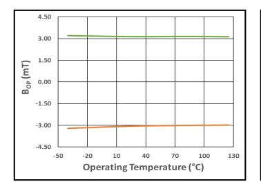
Figure 42.  $B_{OPN}$  (Orange) and  $B_{OPS}$  (Green) vs. Operating Temperature at  $V_{DD}$  = 3.0 V
