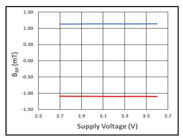
Figure 34.  $B_{RPN}$  (Red) and  $B_{RPS}$  (Blue) vs. Supply Voltage at +25°C
