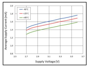
**Figure 44.** Average Supply Current vs. Supply Voltage vs. Temperature
