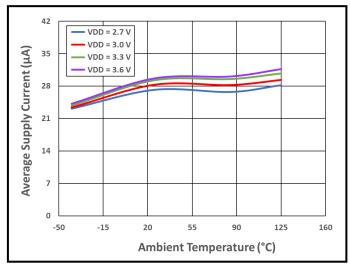
Figure 38. Average Supply Current vs. Temperature vs. Supply Voltage
