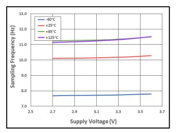
**Figure 14.** Sampling Frequency vs. Supply Voltage vs. Temperature
