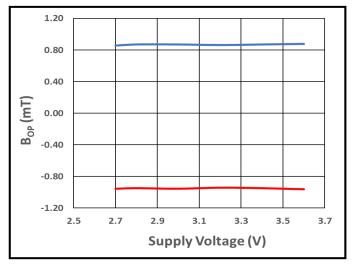
Figure 15.  $B_{\mathsf{OPN}}$  (Red) and  $~B_{\mathsf{OPS}}$  (Blue) vs. Supply Voltage at +25°C
