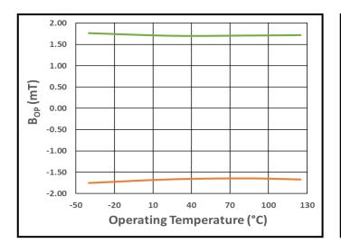
Figure 35.  $B_{OPN}$  (Orange) and  $B_{OPS}$  (Green) vs. Operating Temperature at  $V_{DD}$  = 3.0 V
