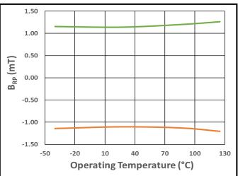
Figure 36.  $B_{RPN}$  (Orange) and  $B_{RPS}$  (Green) vs. Operating Temperature at V<sub>DD</sub> = 3.0 V
