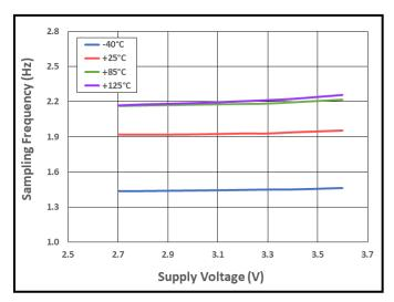
**Figure 7.** Sampling Frequency vs. Supply Voltage vs. Temperature
