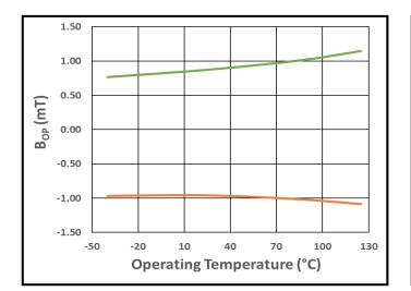
Figure 17.  $B_{OPN}$  (Orange) and  $B_{OPS}$  (Green) vs. Operating Temperature at  $V_{DD}$  = 3.0 V
