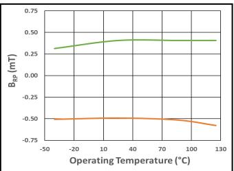
Figure 25.  $B_{RPN}$  (Orange) and  $B_{RPS}$  (Green) vs. Operating Temperature at V<sub>DD</sub> = 3.0 V
