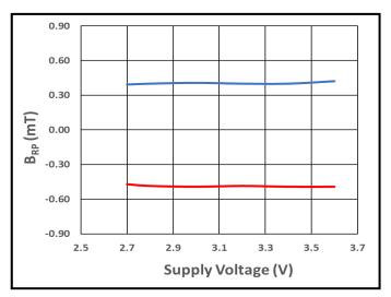
Figure 16.  $B_{RPN}$  (Red) and  $B_{RPS}$  (Blue) vs. Supply Voltage at +25°C
