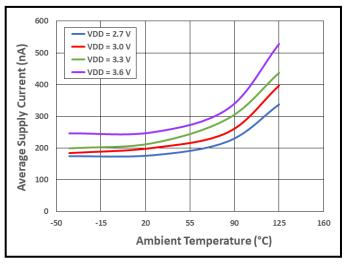
**Figure 6.** Average Supply Current vs. Temperature vs. Supply Voltage
