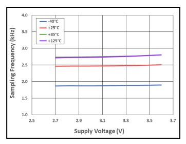
**Figure 32.** Sampling Frequency vs. Supply Voltage vs. Temperature
