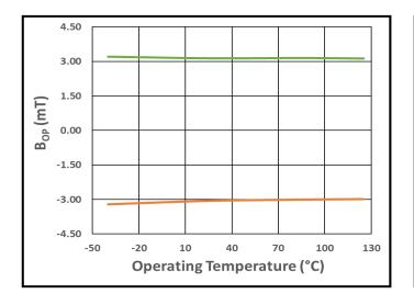
Figure 10.  $B_{OPN}$  (Orange) and  $B_{OPS}$  (Green) vs. Operating Temperature at  $V_{DD}$  = 3.0 V
