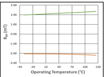
Figure 29.  $B_{RPN}$  (Orange) and  $B_{RPS}$  (Green) vs. Operating Temperature at V<sub>DD</sub> = 3.0 V
