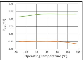
Figure 18.  $B_{RPN}$  (Orange) and  $B_{RPS}$  (Green) vs. Operating Temperature at  $V_{DD}$  = 3.0 V
