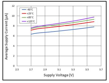
**Figure 30.** Average Supply Current vs. Supply Voltage vs. Temperature
