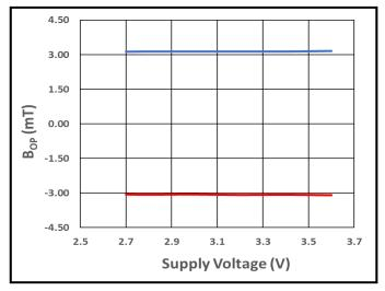
Figure 8.  $B_{OPN}$  (Red) and  $~B_{OPS}$  (Blue) vs. Supply Voltage at +25°C
