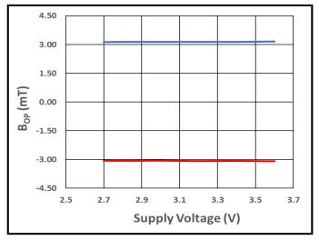
Figure 40.  $B_{\mathsf{OPN}}$  (Red) and  $~B_{\mathsf{OPS}}$  (Blue) vs. Supply Voltage at +25°C
