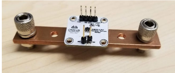
FIGURE 2: CONTACTLESS CURRENT SENSING USING EVB222
