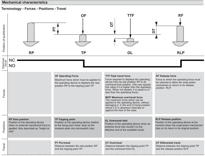
The reference point for the figures given for travel and forces is a point F situated on the button in the case of a plain microswitch, or, generally, 3 mm in from the end of a plain actuator. The reference point for the positions is one of the fixing holes, unless otherwise indicated.
