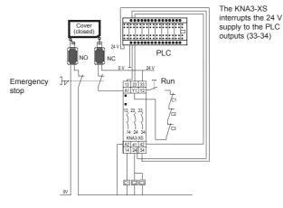
Emergency stop and moving cover controlled by two channels on terminals 41-42 (data contact) to a PLC output.
