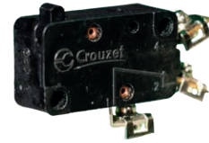
Customised version for nuclear application. Has radiation-resistant housing, 180 °C max operating temperature, W5 screw terminals and magnetic blowout for highly inductive circuit switching at 250 V \overline{-}
