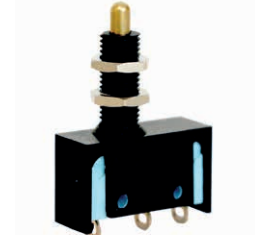
Telescopic plunger with 3 mm overtravel and with M6 x 0.75 threaded barrel
