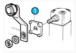
Lever settings or positions dictated by direction in which block 1 is fitted
