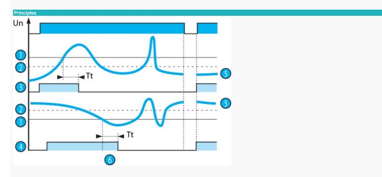
If "with memory" mode has been selected, the relay opens and stays in this position when threshold crossing is detected. The power supply must be disconnected to reset the product.
