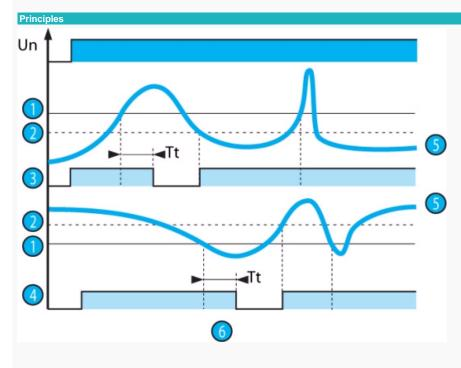
The under or overvoltage threshold value is set by a graduated potentiometer by reading the Un scale to be monitored directly.
