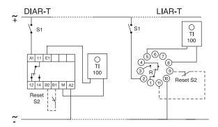
Note: Upon energization of the current control IAR.T Series Relay, the time delay, which is adjustable from .1 to 10 seconds, inhibits the output relay during start-up periods. The delay time is
