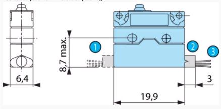
$Black = Common \ Grey = NC \ Blue = NO \ Conductor \ cross-section: 83181 \ / \ 83183 \ / \ 83186 = 0.5 \ mm2 \ 83180 = 0.75 \ mm2$
