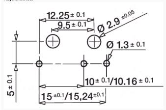
Fixed by 2 M2 screws Torque with screw only: 0.2 Nm, with screw + washer: 0.3 Nm
