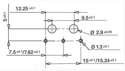
Fixed by 2 M2 screws Torque with screw only : 0.2 Nm, with screw + washer : 0.3 Nm  $\,$
