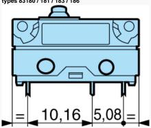
Fixed by 2 M2 screws Torque with screw only : 0.2 Nm, with screw + washer : 0.3 Nm  $\,$
