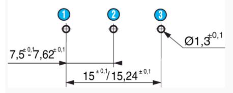
Fixed by 2 M2 screws Torque with screw only : 0.2 Nm, with screw + washer : 0.3 Nm  $\,$
