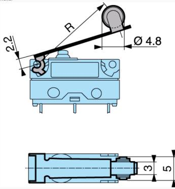
$Black = Common \ Grey = NC \ Blue = NO \ Conductor \ cross-section: 83181 \ / \ 83183 \ / \ 83186 = 3 \ x \ 0.5 \ mm2$
