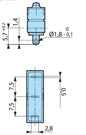
Fixed by 2 M2 screws Torque with screw only : 0.2 Nm, with screw + washer : 0.3 Nm  $\,$
