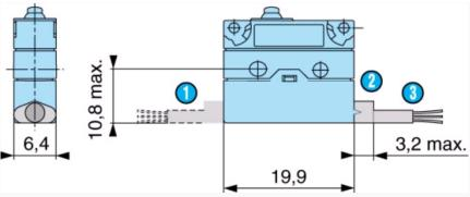
$Black = Common \ Grey = NC \ Blue = NO \ Conductor \ cross-section: 83181 \ / \ 83183 \ / \ 83186 = 3 \ x \ 0.5 \ mm2$
