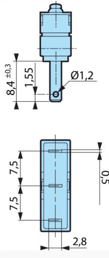
Fixed by 2 M2 screws Torque with screw only: 0.2 Nm, with screw + washer: 0.3 Nm
