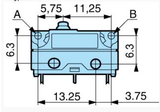
Black = Common Grey = NC Blue = NO Conductor cross-section: 83181 / 83183 / 83186 = 3 x 0.5 mm2
