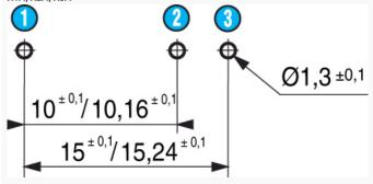
Fixed by 2 M2 screws Torque with screw only : 0.2 Nm, with screw + washer : 0.3 Nm  $\,$
