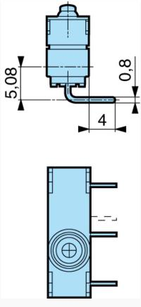
Fixed by 2 M2 screws Torque with screw only : 0.2 Nm, with screw + washer : 0.3 Nm  $\,$
