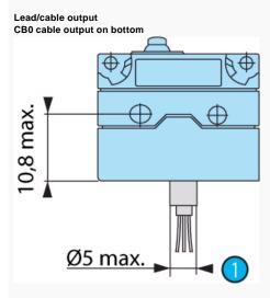
$Black = Common \ Grey = NC \ Blue = NO \ Conductor \ cross-section: 83181 \ / \ 83183 \ / \ 83186 = 0.5 \ mm2 \ 83180 = 0.75 \ mm2$
