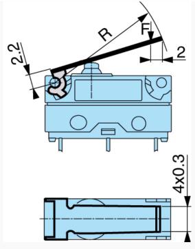
$Black = Common \ Grey = NC \ Blue = NO \ Conductor \ cross-section: 83181 \ / \ 83183 \ / \ 83186 = 3 \ x \ 0.5 \ mm2$
