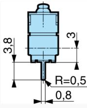
Fixed by 2 M2 screws Torque with screw only : 0.2 Nm, with screw + washer : 0.3 Nm  $\,$
