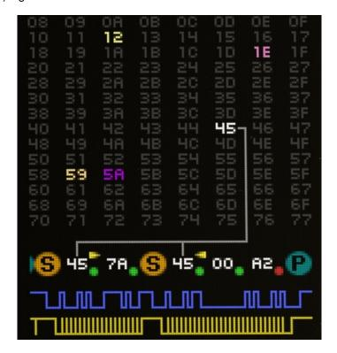
The symbolic decode section shows  $I^2C$  transactions as they happen. Start and stop are shown as (S) and (P) symbols. After a (S) symbol the address byte is shown, with a right arrow (write) or left arrow (read). The gray lines connect the address byte to its heat-map indicator. Following this is a series of data bytes. Each byte is shown in hex, with either a green dot (ACK) or red dot
