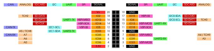
This documents the pinout of the GPIO header, and the default mapping of peripherals when using the Arduino development environment (and other environments with the concept of "board files" follow this layout). Please note that other development environments such as ESP32-IDF and MicroPython provide more flexibility, and allow many of these functions to be mapped to any available pin. However, if compatibility with future add-on boards that work with Arduino is desired, it may make
