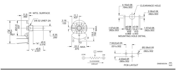
S026 Metal Shaft, Bushing Mounting, Faston Type "S" Formed Terminals
