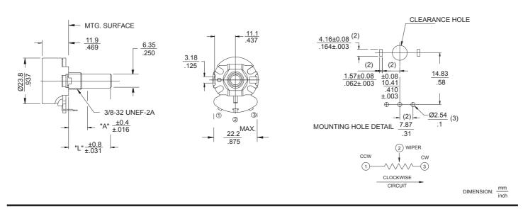
V026 Metal Shaft, Bushing Mounting, Printed Circuit Type "V" Formed Terminals
