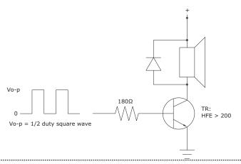
CUI Devices | MODEL: CBT-09427-SMT-TR | DESCRIPTION: MAGNETIC BUZZER TRANSDUCER
