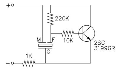
1. The current consumption and the sound pressure level are measured by using the recommended driving circuit shown above. Notes:
