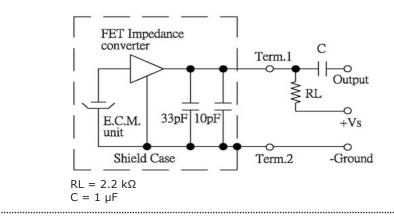
CUI Devices | MODEL: CMC-5042PF-AC | DESCRIPTION: ELECTRET CONDENSER MICROPHONE
