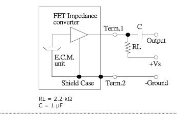
CUI Devices | MODEL: CMC-9745-44P | DESCRIPTION: ELECTRET CONDENSER MICROPHONE
