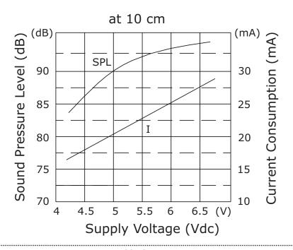
CUI Devices | MODEL: CMI-1265-88-SMT-TR | DESCRIPTION: MAGNETIC BUZZER INDICATOR
