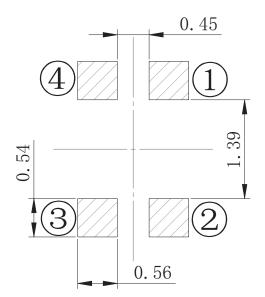
Recommended PCB Layout Top View
