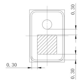
Recommended Vacuum Nozzle Pickup Top View
