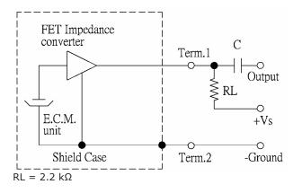
CUI Devices | MODEL: CMR-2747PB-A | DESCRIPTION: ELECTRET CONDENSER MICROPHONE
