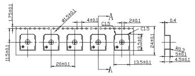
8 positions empty before components, 12 positions empty after components
