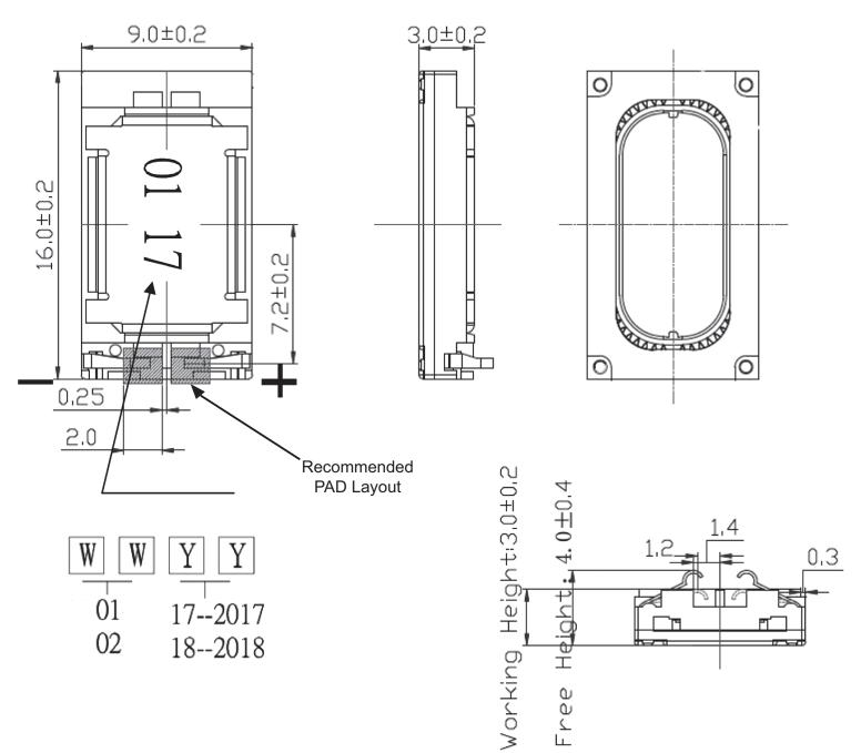
Note: 1. Maximum compression force between front frame and back frame & yoke is 5 N.
