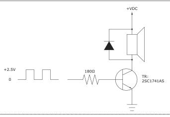
CUI Devices | MODEL: CMT-7525S-SMT-TR | DESCRIPTION: MAGNETIC BUZZER TRANSDUCER
