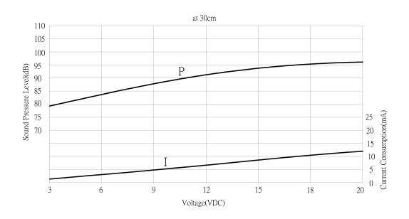
P: Voltage vs. Sound Pressure Level I: Voltage vs. Current Consumption
