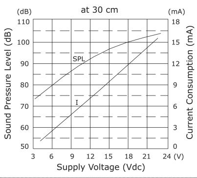
SPL: Voltage vs. Sound Pressure Level I: Voltage vs. Current Consumption
