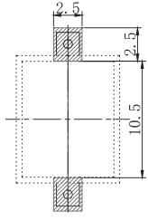
Recommended PCB Layout Top View
