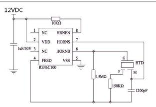
Notes: 1. The current consumption and the sound pressure level are measured by using the recommended driving circuit shown above.
