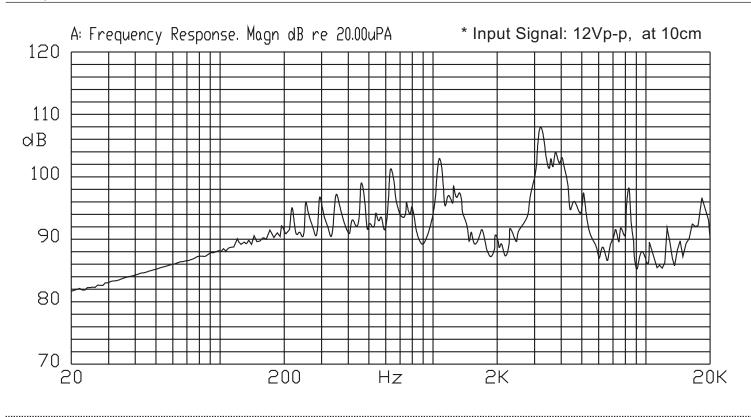
CUI Devices | MODEL: CPT-4011C-600 | DESCRIPTION: PIEZO BUZZER TRANSDUCER
