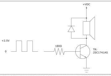
CUI Devices | MODEL: CSS-0575B-SMT-TR | DESCRIPTION: MAGNETIC BUZZER TRANSDUCER
