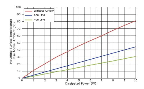
Ths: "hot spot" temperature measured on the heatsink Ta: ambient temperature
