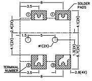
Recommended PCB Layout Top View
