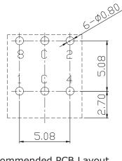
Recommended PCB Layout Top View
