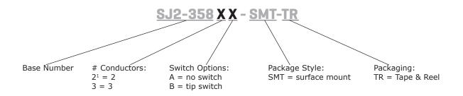
Note: 1. 2 conductor option only available with tip switch
