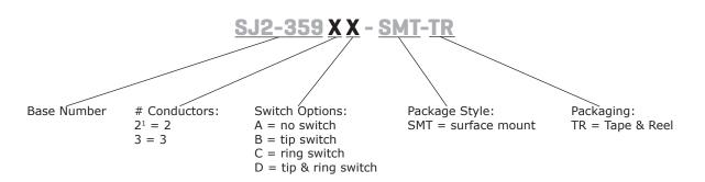
Note: 1. 2 conductor option only available with tip switch
