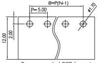
Recommended PCB Layout Top View
