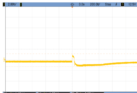
Output voltage waveform (Differential mode 0.90KV)
