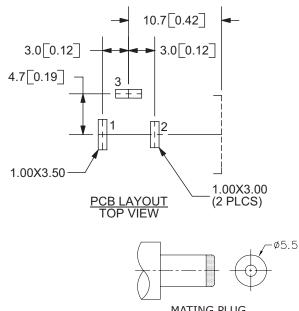
MATING PLUG Jack Insertion Depth: 9.0 mm
